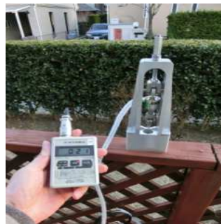
Photo 2 Withdrawal Tool for CMWR
