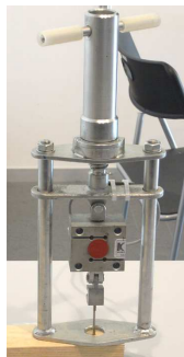
Photo 1 Typical Withdrawal Tool
