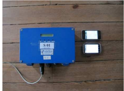
Fig. 2. Calibration of smart phones accelerometers with seismographs.
