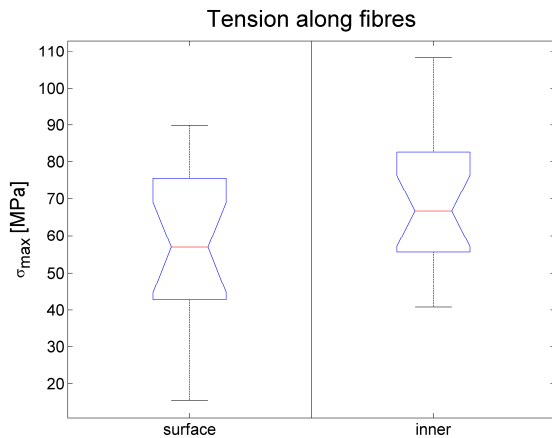
Figure 8: Tension strength along fibres for the surface and the inner part (5×5×7,5 mm)
