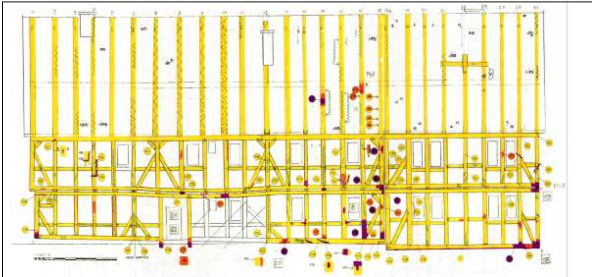
Fig. 6: Example for a simple, combined plan presentation of a half-timbered building. On top of the facade the complete rafter plane of this side is drawn. Such a combination allows for one, the recognition of possible reasons for damage, if, for example, the leaky roof has caused damages to the rafter foot points as well as to the purlin and the post head underneath it in the facade. In individual inventory plans with individual rafter axis and facade drawings, such correlations are often overlooked.
